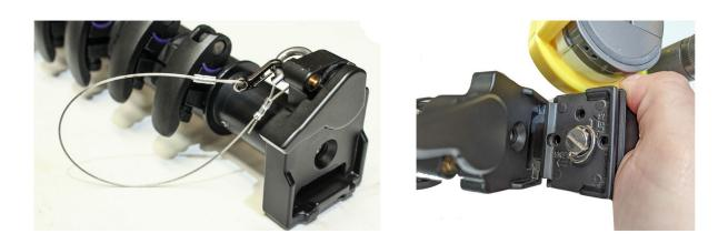
2. Make sute, that safety wire is attached to the Tilt Unit.
