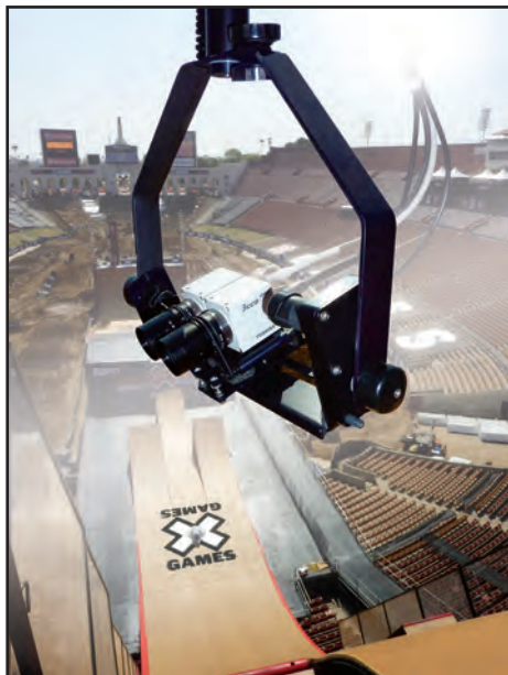
Figure 3. Toshiba Imaging's new IK-HD1 series of high definition cameras on Polecam's compact side-by-side 3D camera rig. (Photo courtesy of Polecam)
