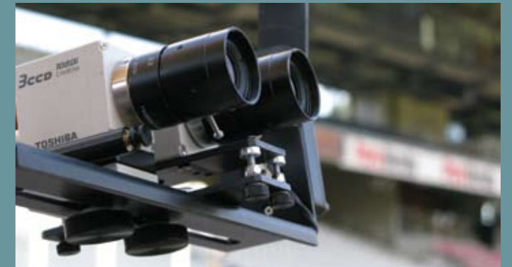
▲ Toshiba IK-HD1E HD 3CCD cameras mounted in 3D-pair configuration on Polecam 3D-Wide head
